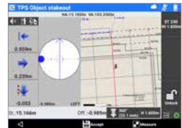
TPS Stakeout in X-PAD Build
