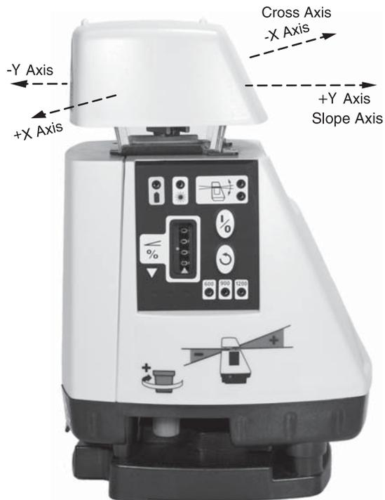
6. The difference between the two marks (if any) is double the difference between how the laser is calibrated and true level for the cross axis. Half way between these two marks is true level. Make a long mark at true level. If the difference between either outer mark and true level is within your working tolerance, go on to step 10. If not, continue with the next step.
