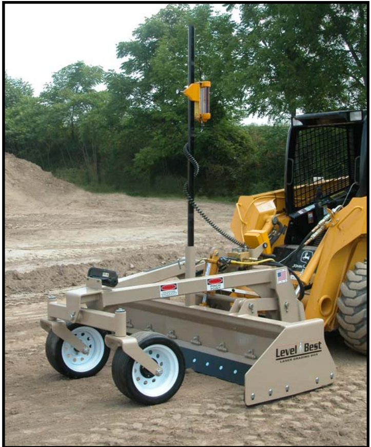
Model PL84 shown with Laser Alignment controls
