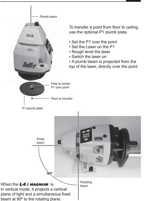
Refer to page 8 for complete instructions on aligning the vertical plane of light. The 90° beam provides a convenient way to define right angle intersections for interior layout.
