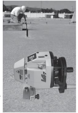
Note: The **L4.7 MAGNUM** laser beam must be rotating with the rotation speed set to maximum when using a receiver.
